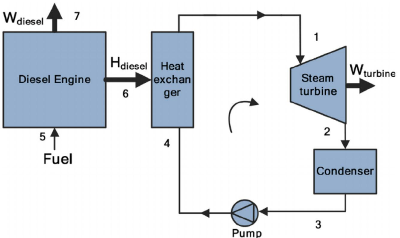
The Rankine cycle (right) is implemented as a closed loop in which the working fluid is chosen to fit the particular needs of the installation. The steam turbine (top right) can be generalised as the 'expander' stage that extracts mechanical energy from the high pressure working fluid.
